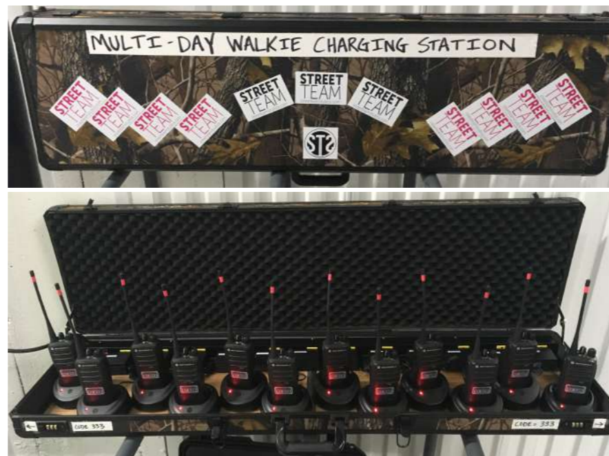
12 Port Multi-Day Charging Station
